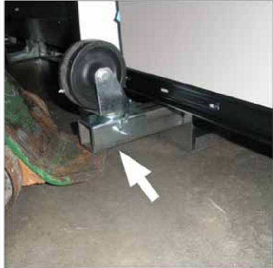
Fig. 2 Using an inverted outrigger as a lifting surface.
